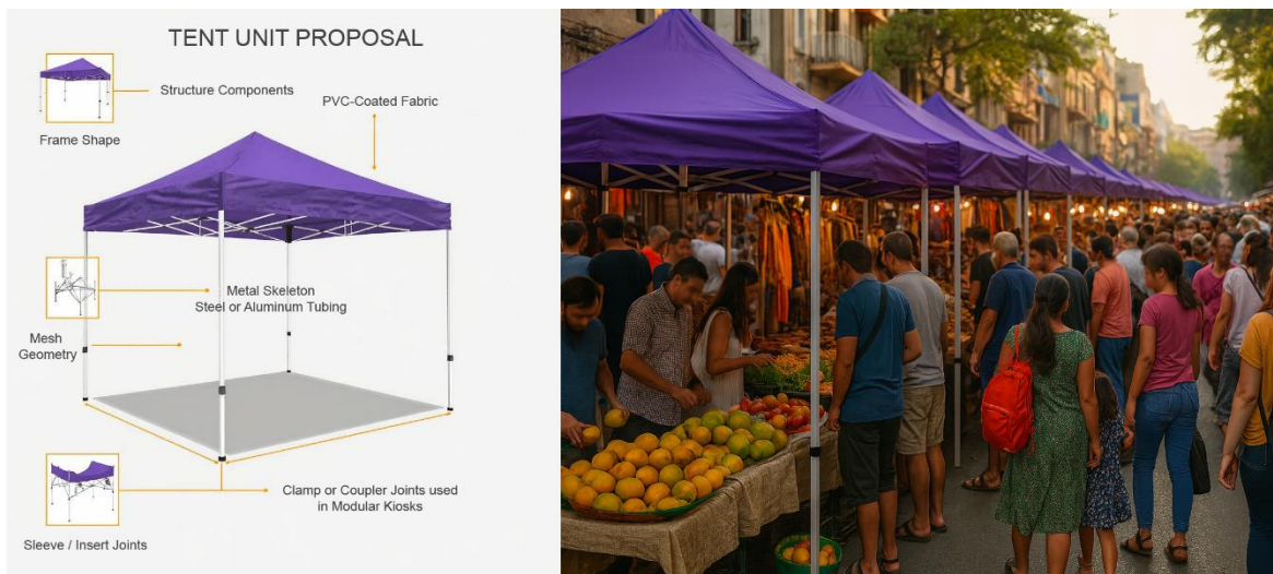
Figure 20: Proposed tent structural visualization.
